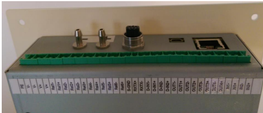
Figure 19: Connection socket for an external HC2 probe
