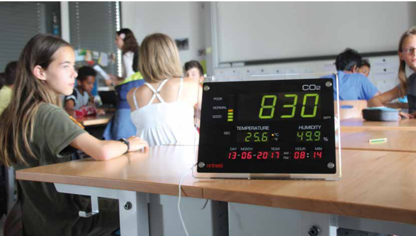
CO 2 display from Rotronic in use in Class 5 / 6B at Köniz-Buchsee Primary School (Switzerland).
