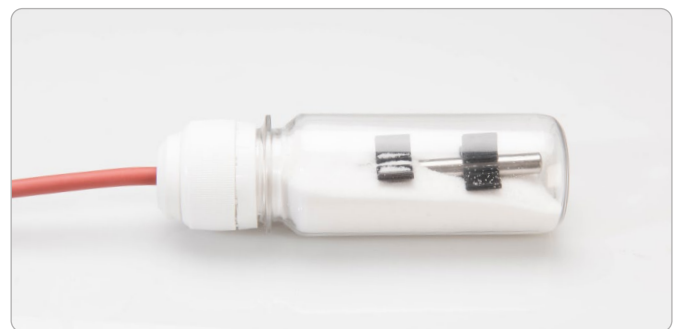
Centering sleeves in situ
